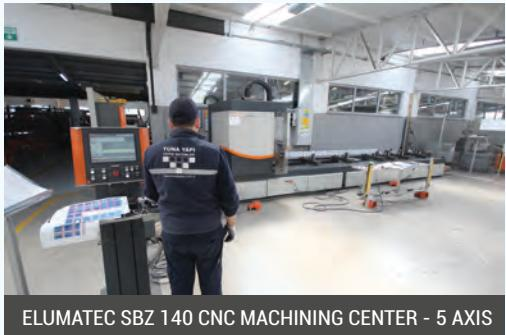
ELUMATEC SBZ 140 CNC MACHINING CENTER - 5 AXIS
