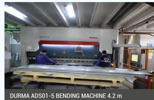
DURMA ADS01-5 BENDING MACHINE 4.2 m
