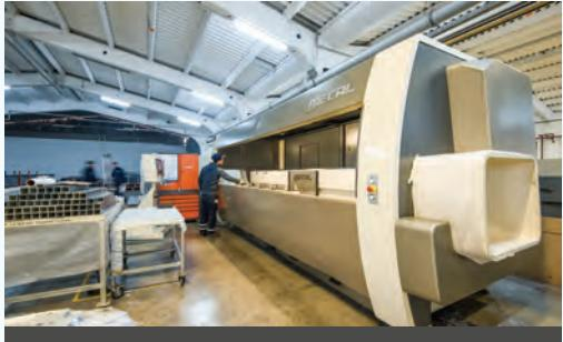
MECAL FALCON CNC MACHINING CENTER - 4 AXIS
